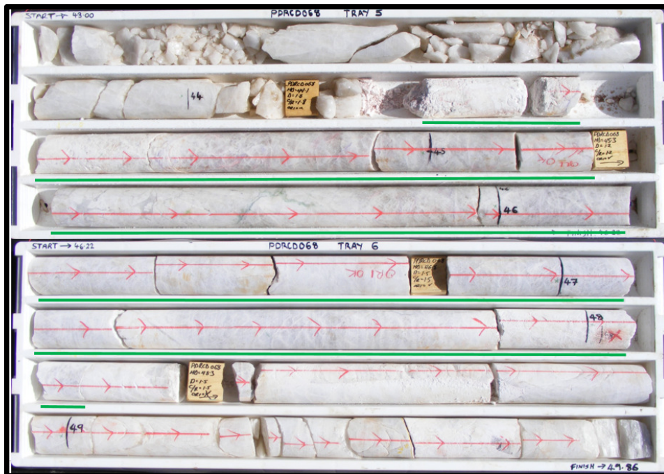
Photograph 1. From diamond core hole PDRCD068, located 10m north of discovery RC hole PDRCD015. Pioneer's geologists have logged the interval between 41.15m and 48.13m ( highlighted in green ) as being predominantly pollucite.
